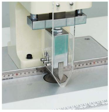
Free located cutter rest, with dividing ruler which can measure the cutting length conveniently
